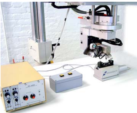
X-ray elastic constant determination system.
