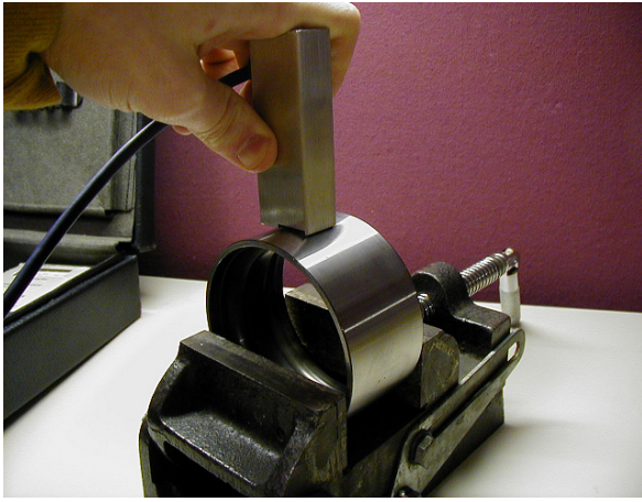
Figure 5 – Handheld testing of bearing ring using OD sensor.
