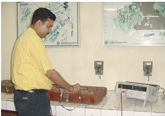
An engineer from Adtech evaluating residual stress on CI engine blocks at customer's place with Stresscan 500.
